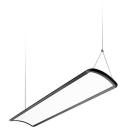
CURVELYTE 1265x330 HO D/I 3K DALI BLACK is a suspended LED Linear luminaire with Direct / Indirect (70/30) distribution. Luminaire Dimensions: 1265x336x46mm, Black body colour, IP20, IK06. Constant Current, Low LED flicker (<5%), Warm White (3000K) LED Colour Temperature, 6250lm, 55W, 114lm/W efficacy, CRI>80, 3 SDCM (3-step MacAdam ellipse) LED Colour Consistency, Lifespan 49,000 hours L80B20, Terminal block connection in the driver box. Glow Wire Test 650°C.
